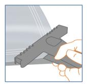
**8.** Diagonally seal across all four corners of the CadSeal foil to re-enforce the corner seals.
