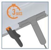
**6a.** Seal the foil together by holding the heat sealer on the foil for approximately 3 seconds.
