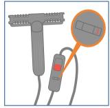
**1.** Plug the sealer into power. Slide the switch to position three. It will take approximately 10 minutes to heat up to 125°C/257°F.
