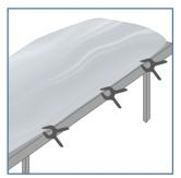
**5.** Use the clamps provided in starter kit, to hold the two pieces of foil together.
